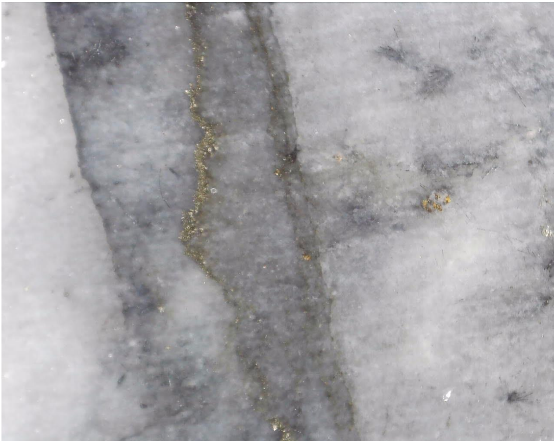
Photo 2: SDDSC050 713.9 m showing visible gold associated with and adjacent to pyrite veinlets within quartz carbonate vein. Field of view 7 mm.
