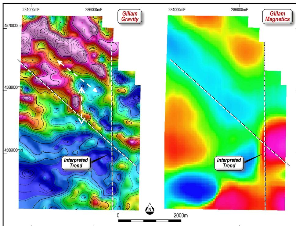
**Figure 2:** Results from recent Gillam gravity survey (left) compared with the magnetic survey (right).
