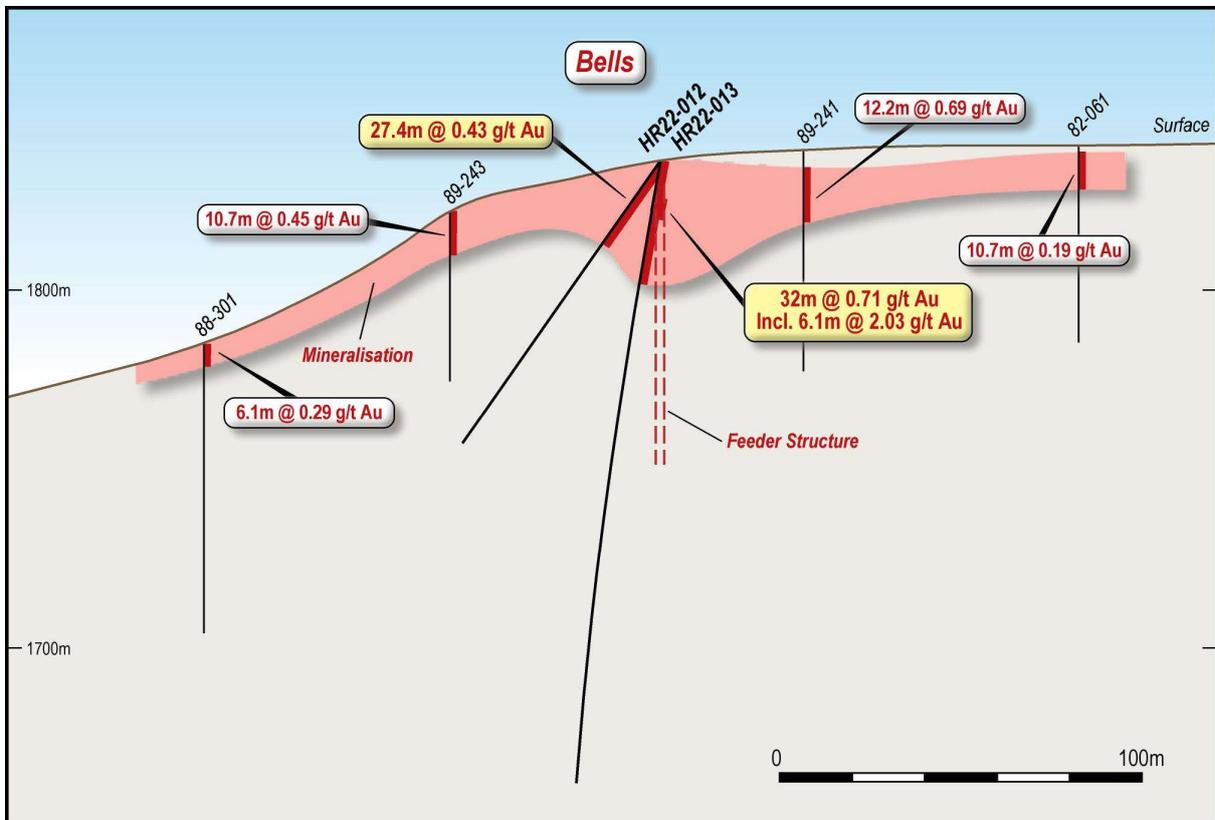
Figure 5: Bells cross section highlighting the interpreted location of a controlling mineralised fault which cuts through the central position of the Bells Project in a north-west direction.
