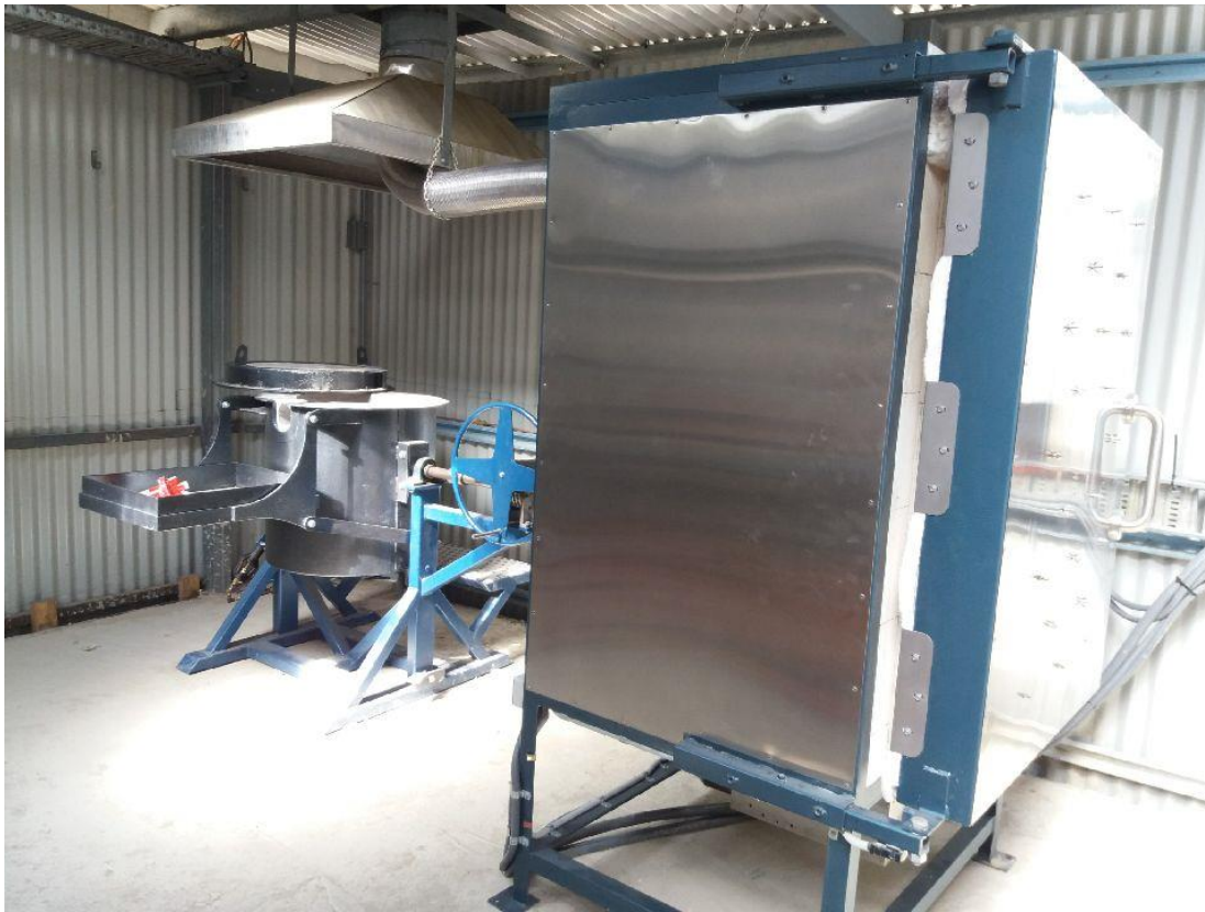
Figure 6 – Gold Room at Woods Point with new Calcining oven in the foreground, and the Furnace towards the back.
