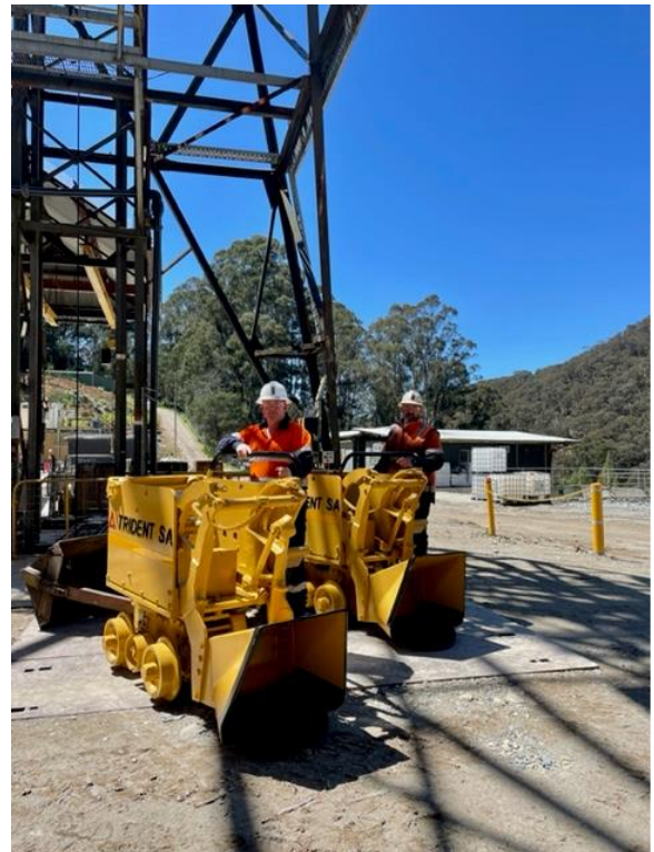
Figure 3 – New 12B bidders prior to commissioning underground.
