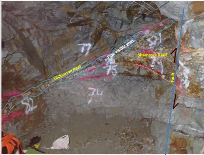
Figure 4 - Face showing the contact between Dickenson Reef (left), fresh, grey quartz and rusty brown broken Shamrock (right).
