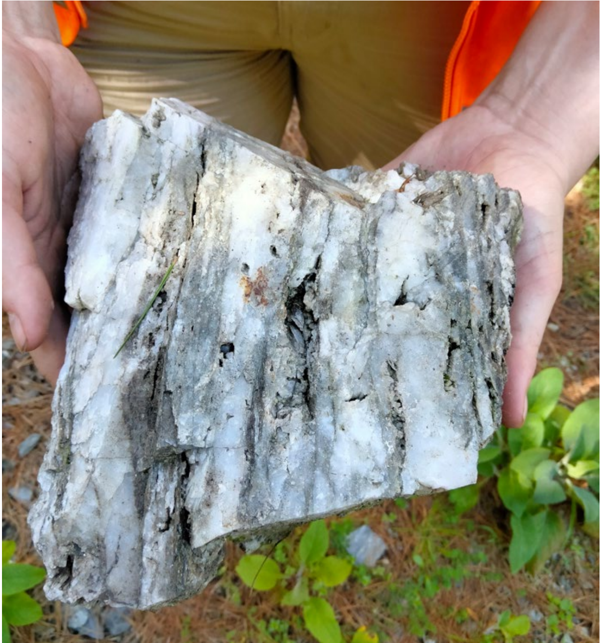
Figure 3 - Weathered Golden Bar Quartz vein showing ribbon banded quartz textures with diffuse wall rock inclusions and some stylolitic planes. This vein texture is typical of high-grade mesothermal orogenic gold deposits
