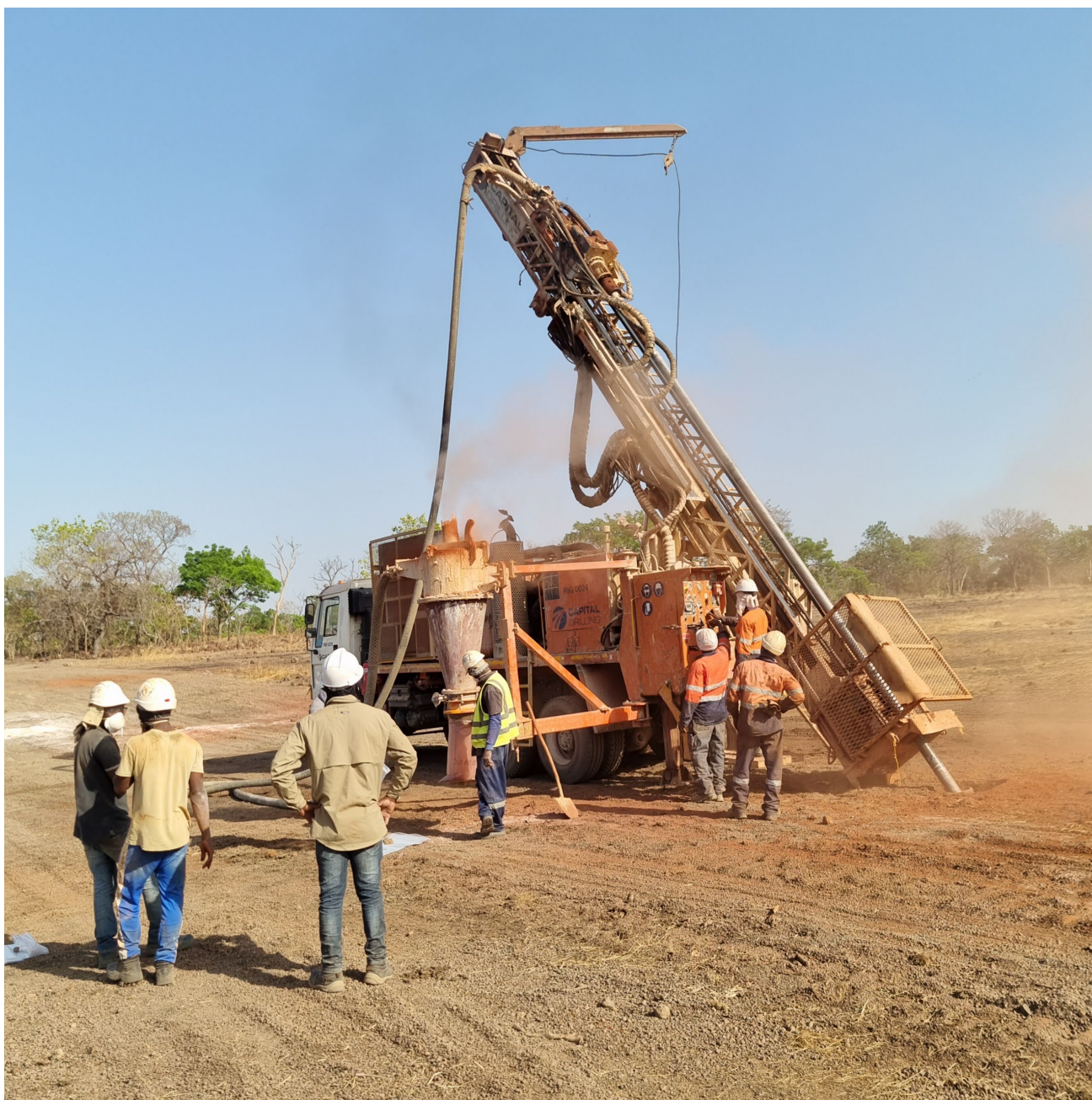
Figure 1: First hole of the 5,000m AC drilling program at Kada Gold Project, Guinea
