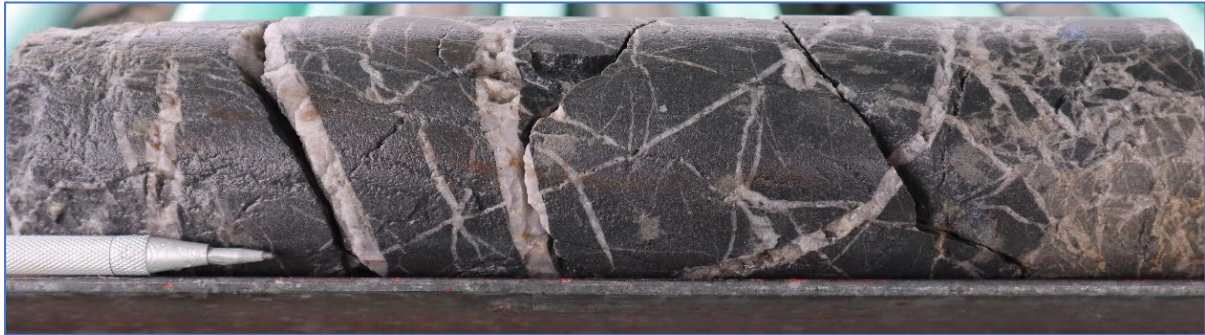
Figure 4: Core with pyrite bearing network veins & vein infill breccia hosted in phyllic altered sandstone - PPDD001 at 47.2m
