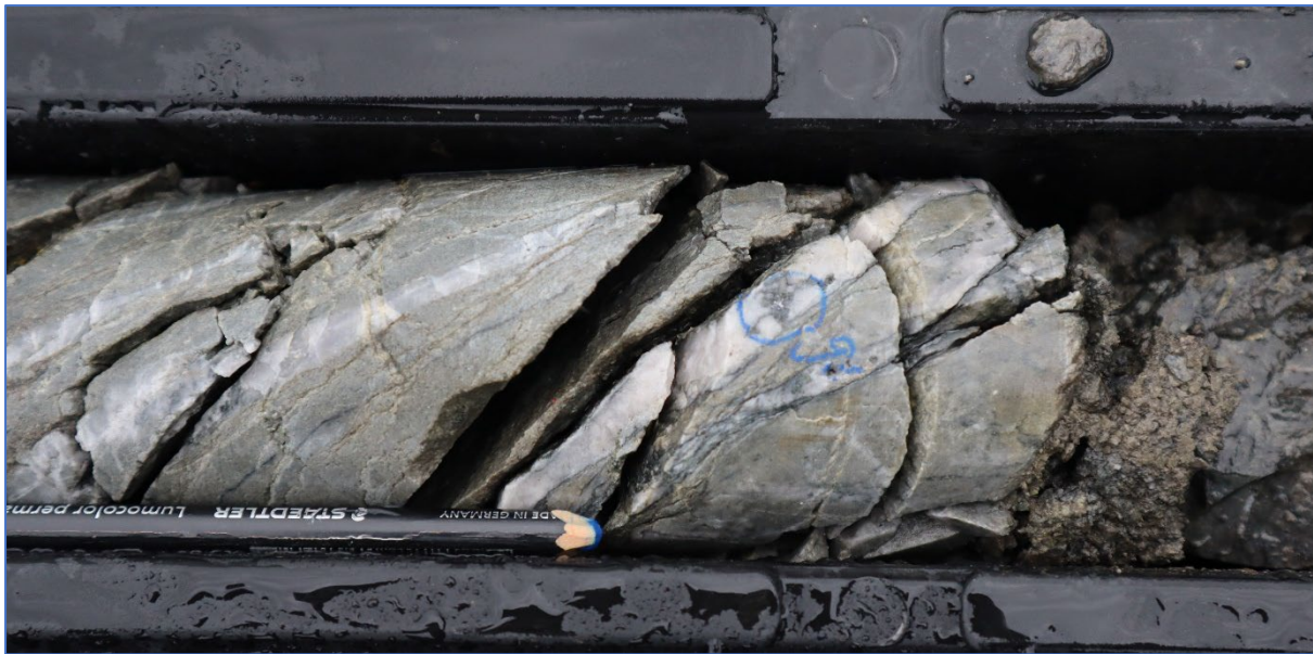
Figure 7: Sheeted quartz veining bearing galena with fine-grained arsenopyrite hosted in intensely phyllic altered sandstone - PPDD002 at 38.40m
