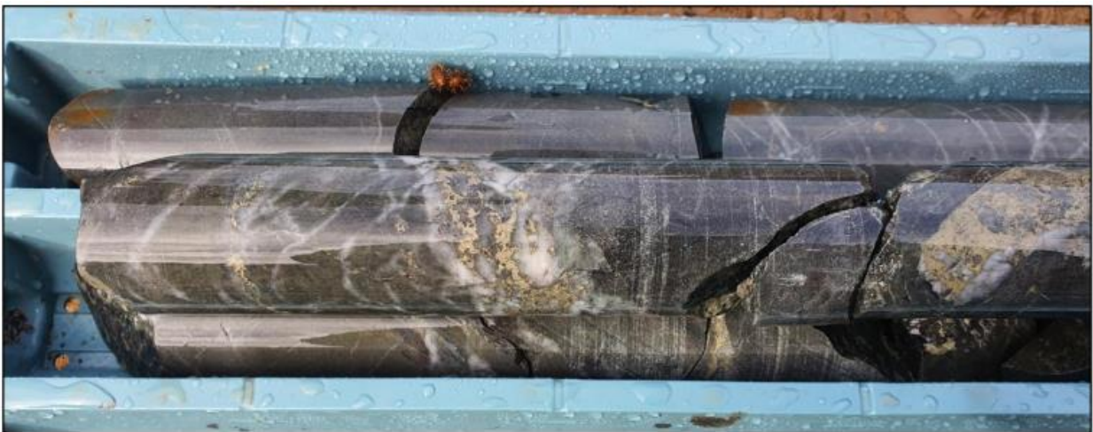
Figure 8: A chlorite-epidote altered chalcopyrite sulphide quartz vein overprinting potassic biotite-magnetite veins from 322m in Hole 4
