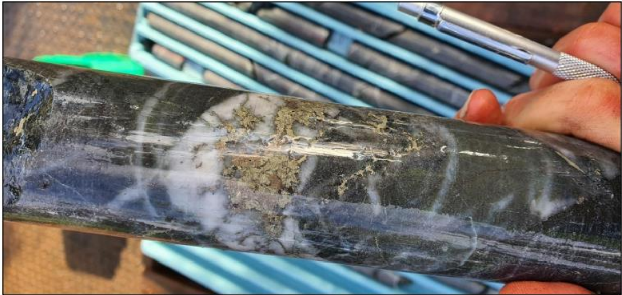
Figure 7: Chalcopyrite + Pyrite + Quartz veins from Hole 4 @ 322.5m
