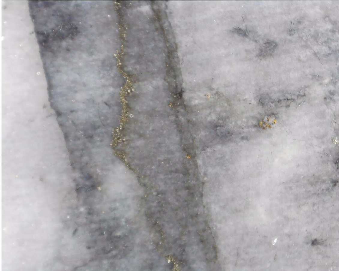
Photo 2: SDDSC050 713.9 m showing visible gold associated with and adjacent to pyrite veinlets within quartz carbonate vein. Field of view 7 mm.
