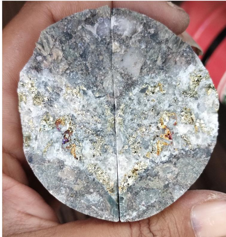
Figure 2: Disseminated bornite (copper iron sulphide) in calcite vein – FI2405 at 376 metres.
