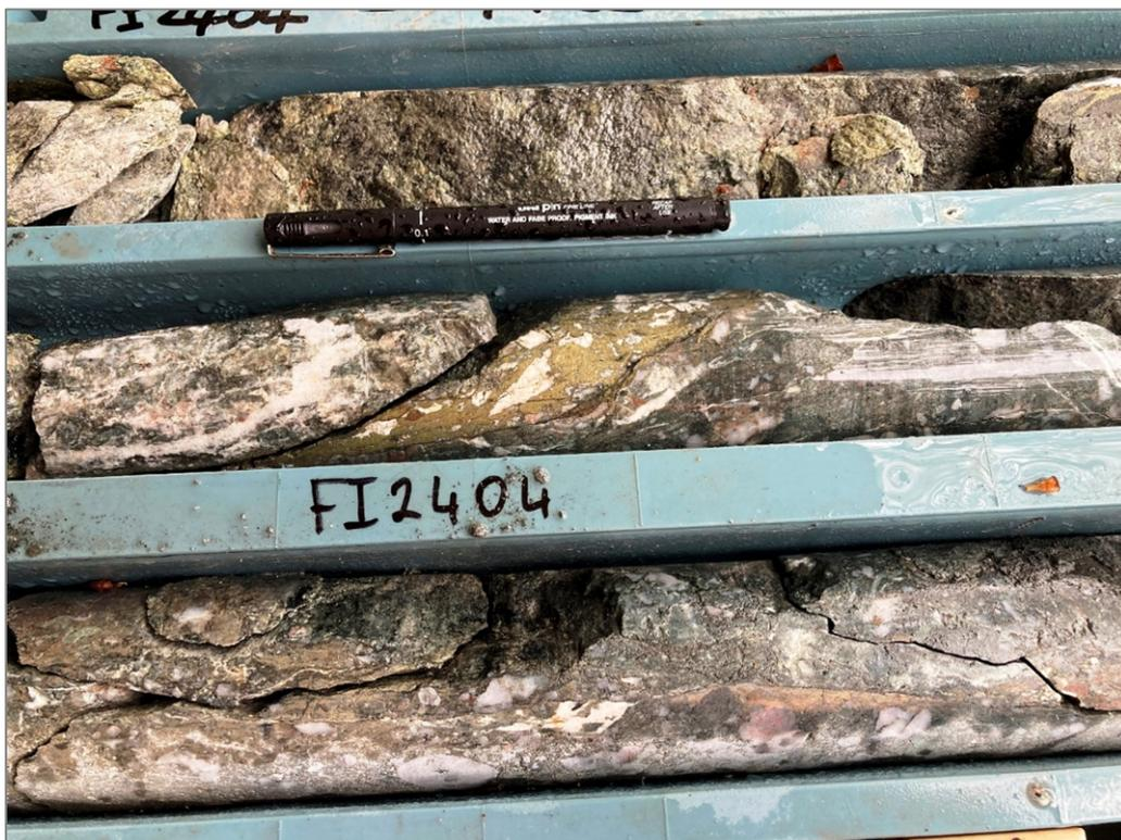
Figure 3: Stringer chalcopyrite (copper sulphide) in chloritic shear zone – FI2404 at 511 metres.
