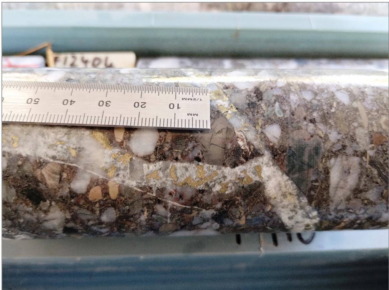
**Figure 1: Coarse-grained blebby sulphide (chalcopyrite) in calcite vein – FI2404 at 469.4 metres.**
