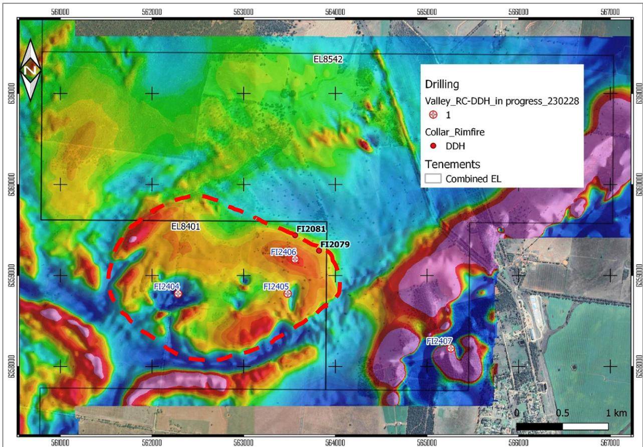
**Figure 7: Valley magnetic image showing drill hole locations, and discrete magnetic anomalies within a broader “ring” feature potentially indicative of buried intrusive rock complexes.**
