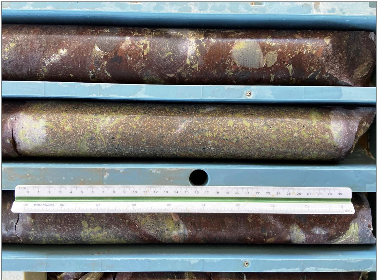
**Figure 4: Epidote (green) and hematite (red) altered andesitic volcanic rock of the Raggatt Volcanics – FI2404 at 600 metres.**
