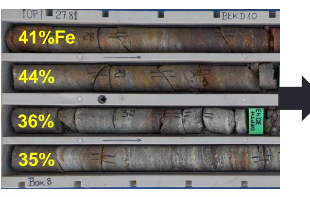
Bekisopa Drill Core BEKD10 Upgrades to 70% Iron 0.5% SiO<sub>2</sub>, 0.7%Al<sub>2</sub>O<sub>3</sub>, 0.003%P & 0.004%S "Super" Premium Grade Iron Concentrate at 75-micron 44% DTR
