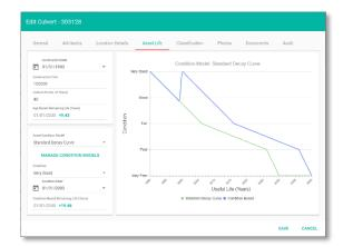
To help with broadly estimating the condition of physical assets over time, various industry bodies have put together deterioration/decay curves that plot the expected condition of a certain type of asset over its typical "useful life".
