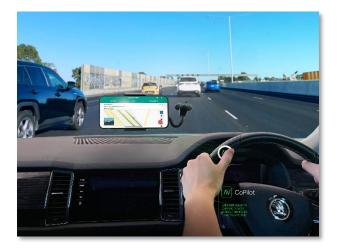
Asset Vision's innovative CoPilot solution enables road inspectors to inspect the roads and capture defects efficiently and safely without taking their hands off the steering wheel.
