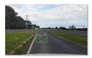
AutoPilot+Al uses a cutting-edge Al model that has been trained on a large amount of data to detect potholes in real-time.
