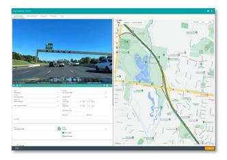
AutoPilot enables our mobile app to automatically and silently capture photos of the oncoming road every 10 metres during an inspection.
