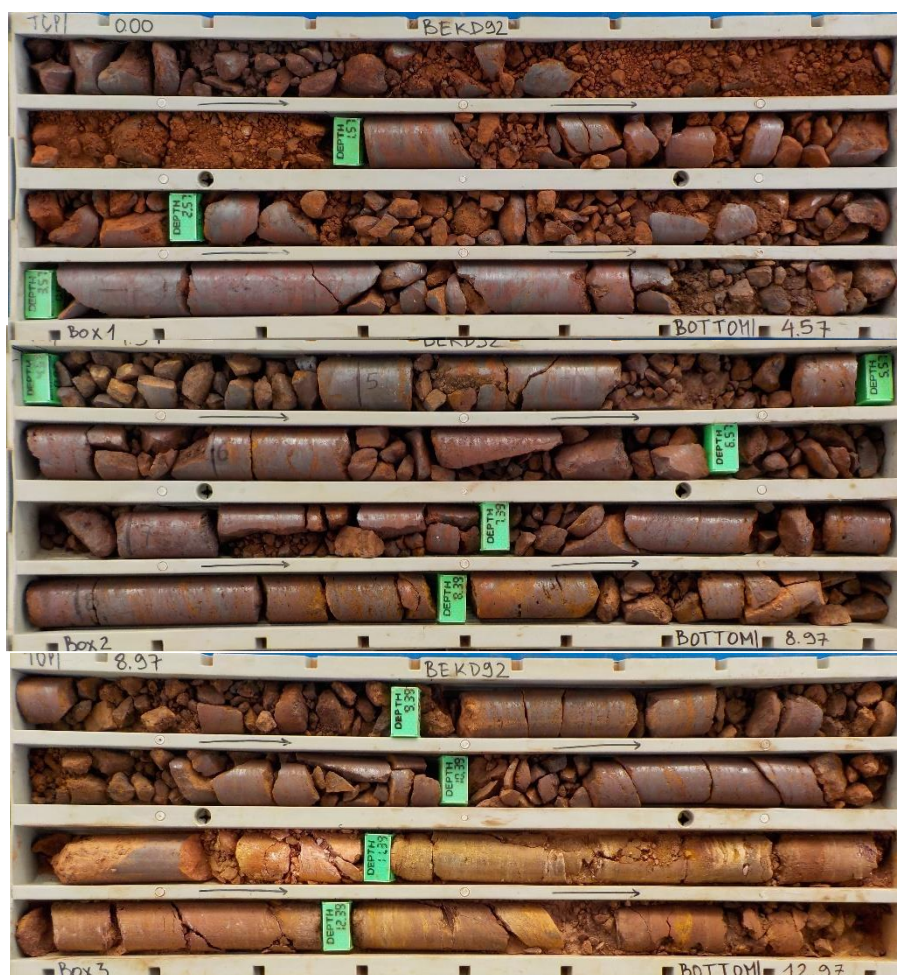
Figure 5(b) 2022 DSO infill drill core from drill hole BEKD092, showing potentially high-grade DSO lump and fines iron ore product grading 66% Fe, from surface to 11.2m
