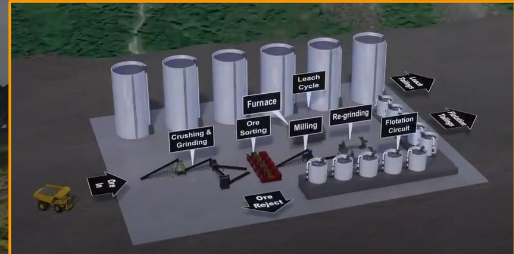
Proposed Estelle central processing plant
