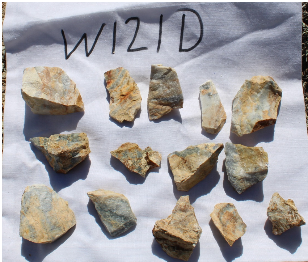
Figure 4. Photo of mine dump sample W121 from the main Warrior Mine dump - 17.55g/t Au, 57.4g/t Ag, 525ppm As, 71.75ppm Sb & 6.88ppm Hg . Crudely banded dark matrix sulphide with crystalline quartz, marcasite and pyrite. Au/Ag ratio = 0.31.
