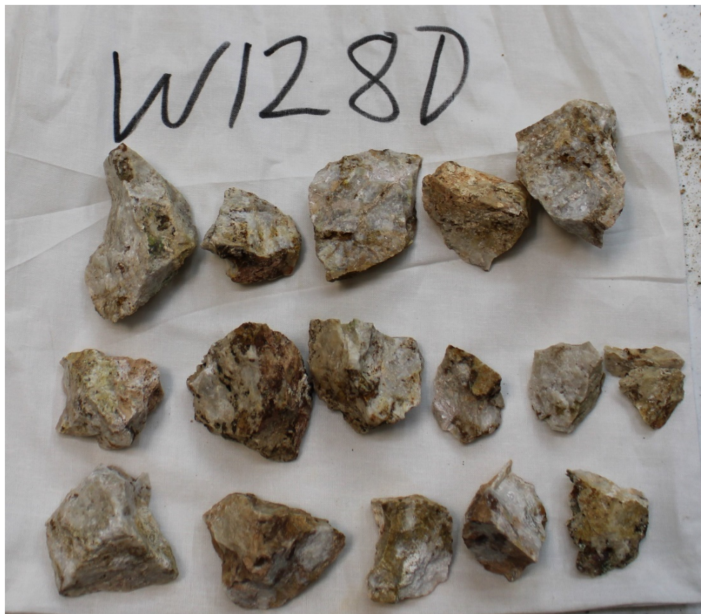
Figure 6. Photo of mine dump sample W128 from the Hillside Mine dump which returned 23.2g/t Au, 15.15g/t Ag, 266ppm As, 38.8ppm Sb & 1.43ppm Hg . Bladed to massive quartz vein material showing some minor weakly developed banding. Au/Ag ratio = 1.5.
