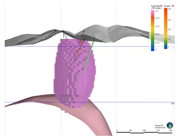
Figure 3 - North Scamander Prospect Cross Section (looking NW) – Proposed drillhole NSD005, Historic drillholes with tin grades, modelled granite surface (pale pink) and Magnetic Inversion (0.015 to 0.59 x10^-5 SI units) (bright pink)
