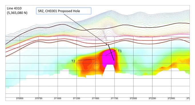
Figure 7 – Carbine Hill East Prospect Cross Section, Flight Line 4310 (5,365,080 N) Resistivity Depth Image (RDI), Surface Topography (brown line), EM TAU dB/dt Z Profile (above topography), Modelled Plates and Proposed Drillhole (Source: EL22/2010 Yunnan Tin 2015 Annual Report, Appendix 5)
