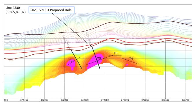
Figure 9 - Evenden Prospect Cross Section, Flight Line 4320 (5,365,890 N) - Resistivity Depth Image (RDI), Surface Topography (brown line), EM TAU dB/dt Z Profile (above topography), Modelled Plates and Proposed Drillhole (Source: EL22/2010 Yunnan Tin 2015 Annual Report, Appendix 5)
