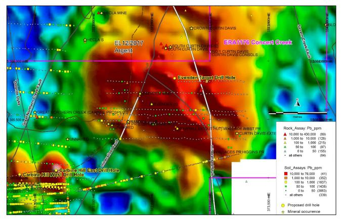
Figure 8 - 2013 VTEM Ch45 anomalies with historic rock chip and soil results for Lead, historic mineral occurrences and EL29/2022 Drill Targets
