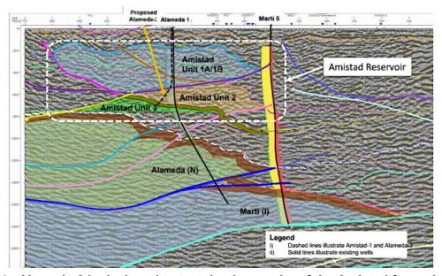
Figure 4 - Alameda-2 is designed to test the three units of the Amistad formation
