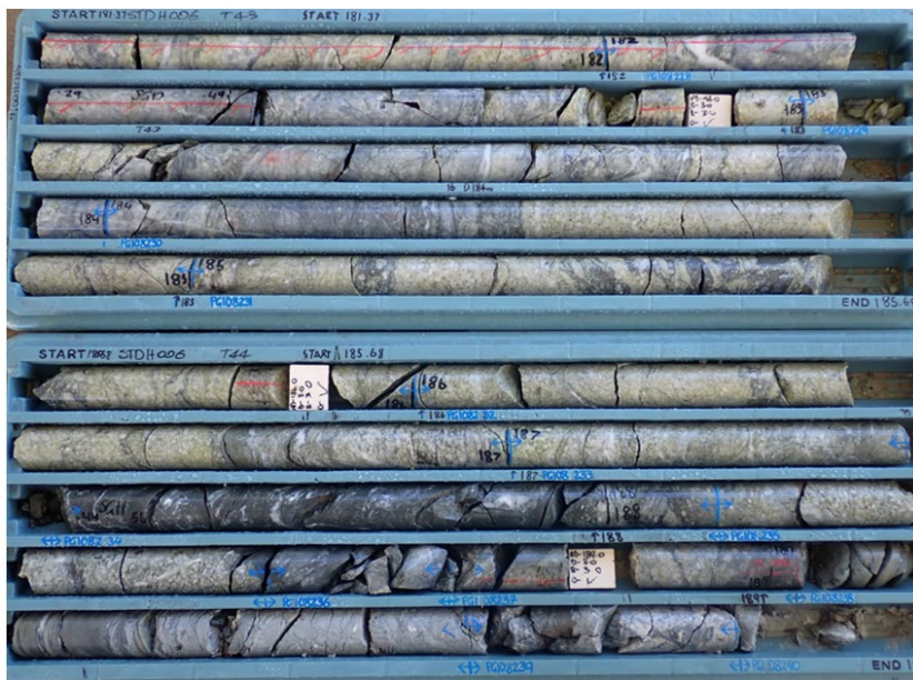
Figure 3: STDH006 drill core showing strong veining and alteration associated with an IP target concealed by shallow cover and highlighting potential to link the main Southern Target gold systems over >1.8km (results pending). Core shown from 181.4m to 189.9m forming a portion of the 50m downhole zone of veining and alteration.
