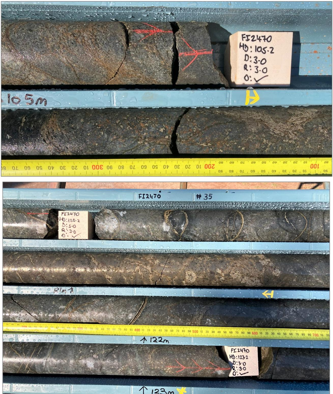
Figure 1: Stringer and heavy disseminated sulphides at 105 metres in FI2470 (upper photo). Massive and strongly disseminated sulphide mineralisation at 121 – 123 metres in FI2470 (lower photo).
