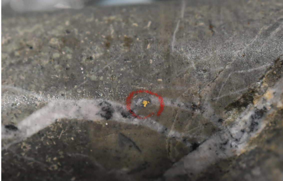
Photo 6: SDDSC064 between 890.2-890.7 m showing visible gold within a quartz carbonate vein hosted by albitised and sericitized dioritic dyke. Drill core (NQ) is 47.6 mm wide
