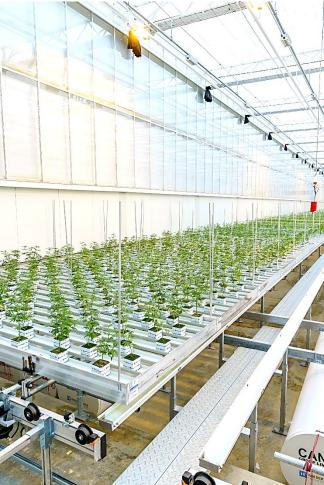
Automated plant movement conveyors and plant propagation systems
