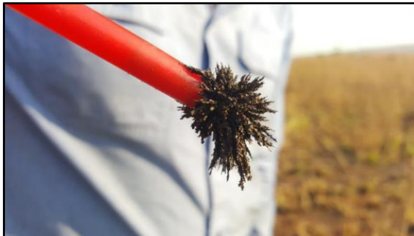
Photo 5.2: Magnetite Particles on Hand Magnet from Red Soil
