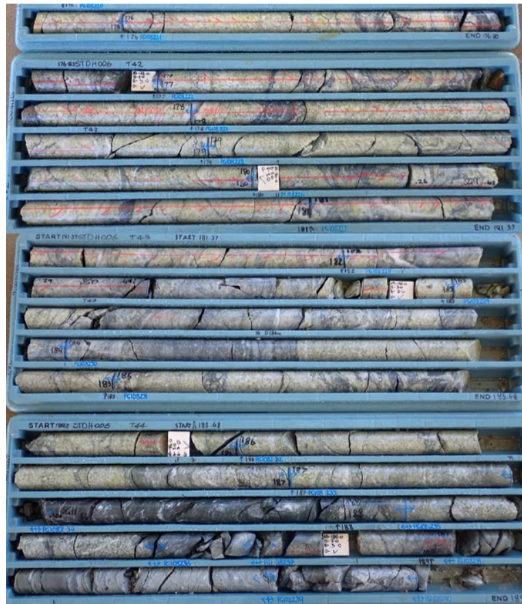
Figure 3: STDH006 drill core showing strong veining and alteration associated with an IP resistivity target which intersected broad gold mineralisation including 26.8m @ 0.6g/t Au from 176m
