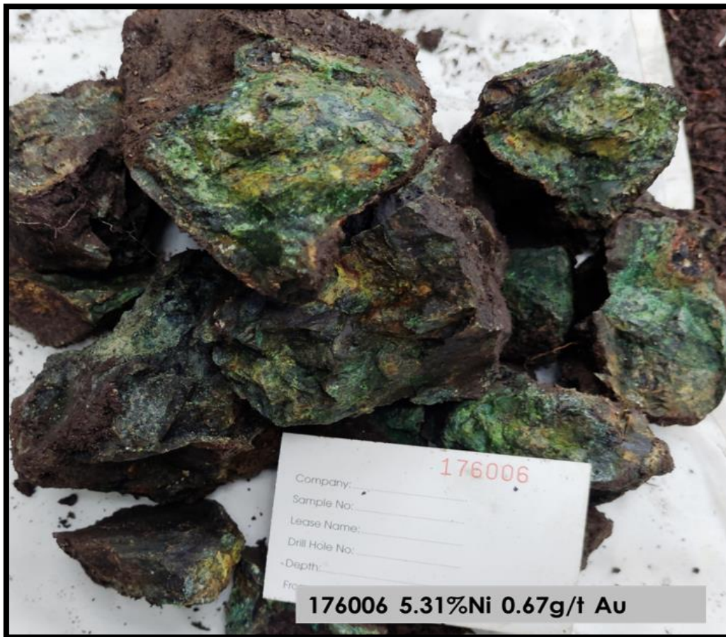
Plate 3: Sample 176006 from trench FPR T1 which assayed 5.31% Ni and 0.67g/t Au. The sample was taken from a scout pit dug within the corridor and contains garnierite and nickel sulphide minerals. See Figures 2 & 3.
