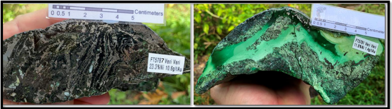
Plate 2: Examples of high grade nickel boudins. Note the curved outer surface, which is typical of boudins formed in shears. The high grade nickel sulphide mineral assemblage is typical of low Fe and low S bearing fluids associated with serpentinisation of ultramafic rocks. Garnierite (vibrant green Ni-Silicate in right photo) is typically found in association with the nickel sulphide and serpentinised shears 3 .
