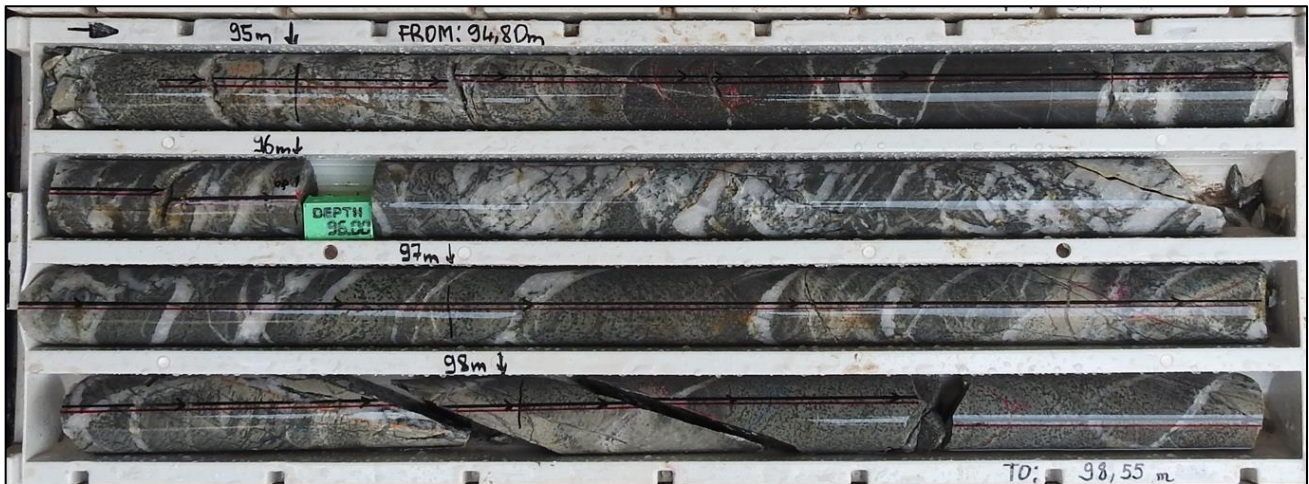
Figure 2: MSDD014 drill core showing area of weakly sheared greywacke, with intense veining and local wall rock hydrothermal brecciation. Breccia consists of monomictic subangular fragments hosted in a pyrite rich, quartz-carbonate stockwork.
