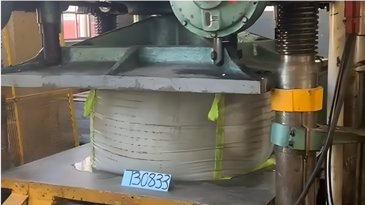
Compression testing of geotextile backfill bags containing ATA™ solids
