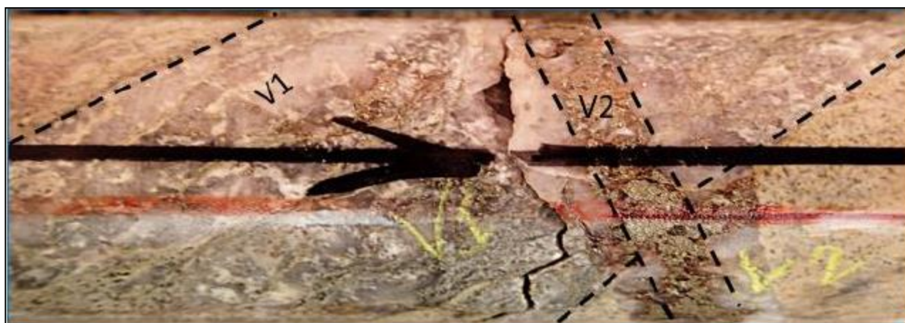
Figure 4: Thin pyrite-rich V2a vein crosscutting obliquely a quartz-carbonate-pyrite V1 vein, MSDD007, 260 m.
