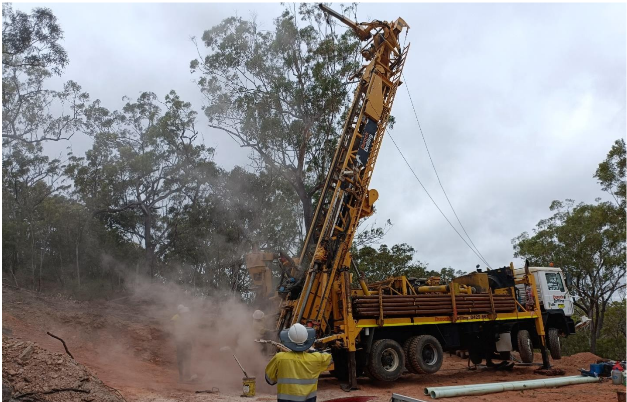
Figure 1: Durock Drilling UDR 1200 RC Drill Rig at Orient West
