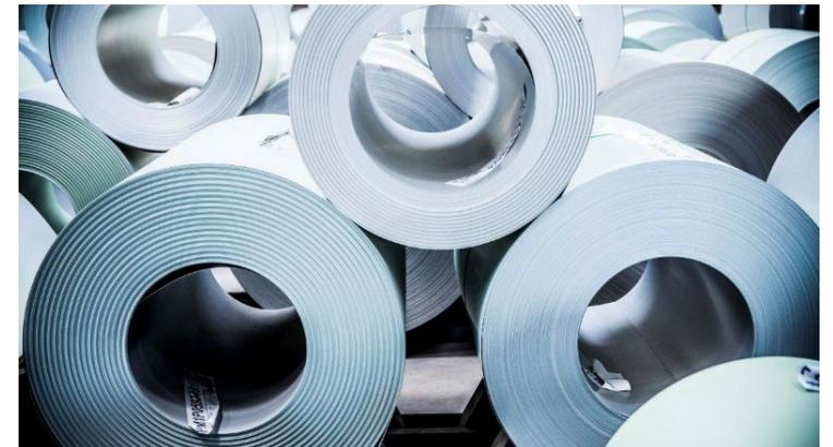
1. AM coating: Introduces magnesium into aluminium-zinc alloy (AZ) coating, which improves galvanic protection over AZ coating by activating the aluminium AZ coating: Steel with a protective alloy coating of zinc and aluminium to protect its steel base against corrosion.
