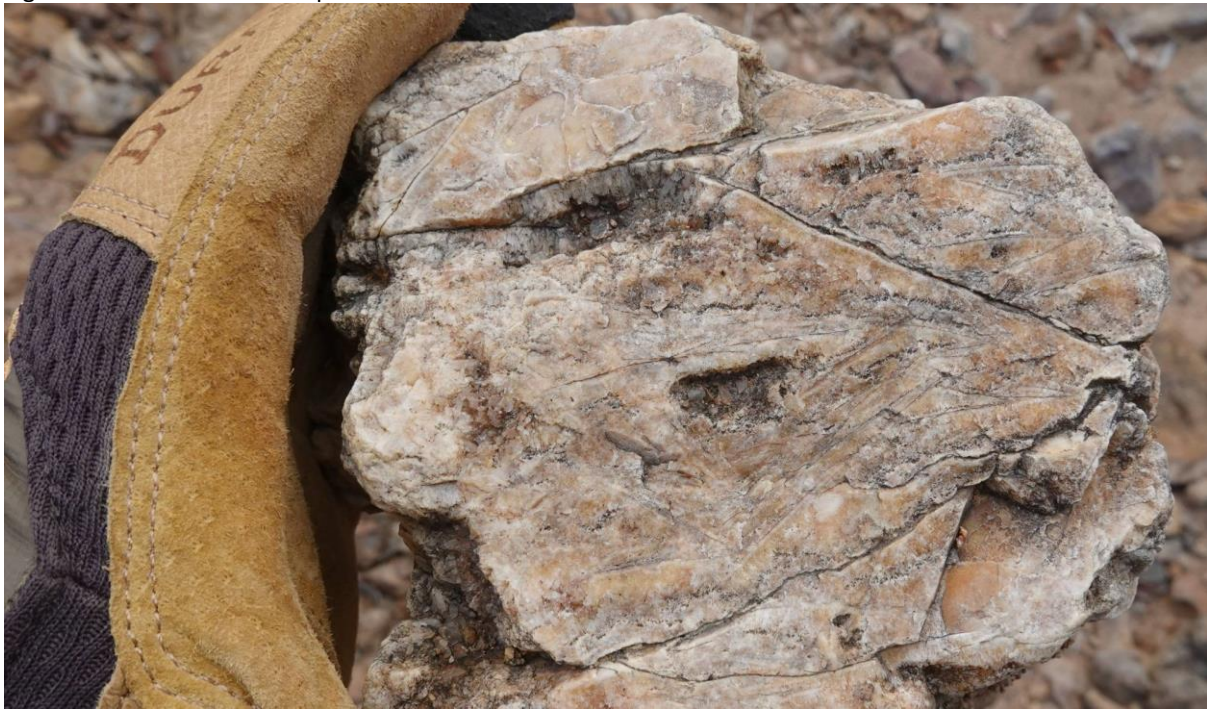
Figure 7 Bladed carbonate replacement texture
