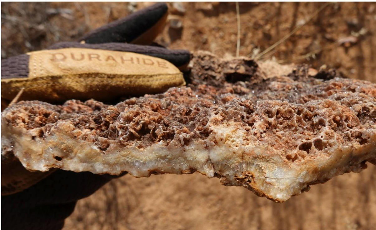
Figure 10 Sulphide boxworks in colloform banded quartz
