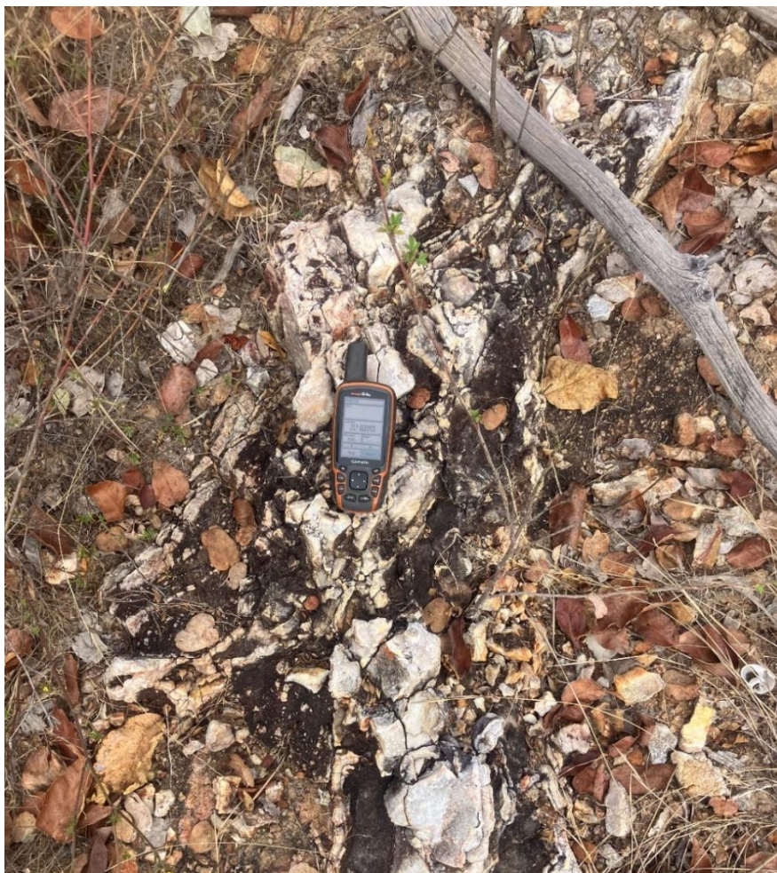
Figure 1 Epithermal Quartz Vein: BM025 sample returned 7.85 g/t Au & 2.17 g/t Ag
