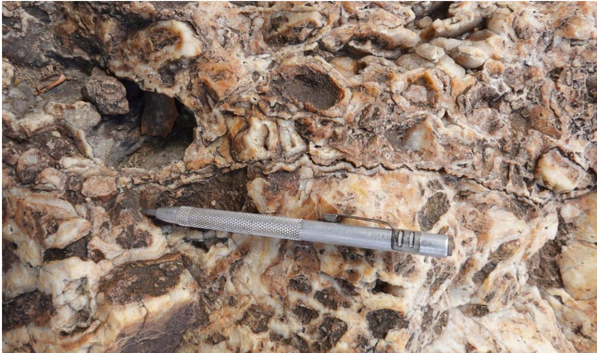
Figure 9 Breccia pod detail with gossan bands
