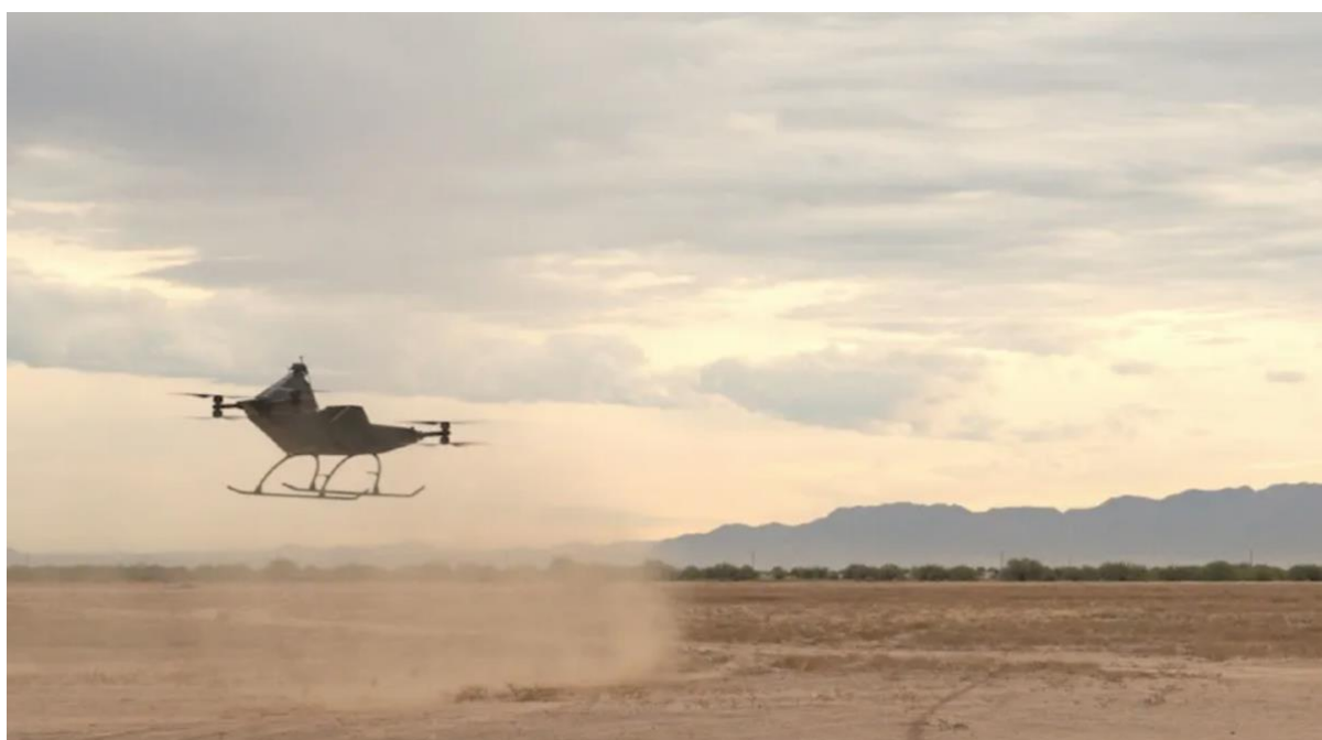
Figure 1. Fully electric DRAGON eVTOL Personal Air Vehicle (PAV) from Rotor X undergoing test flights in the Arizona desert recently
