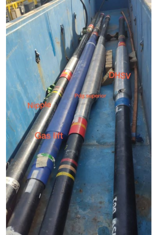
Upper Completion Equipment
