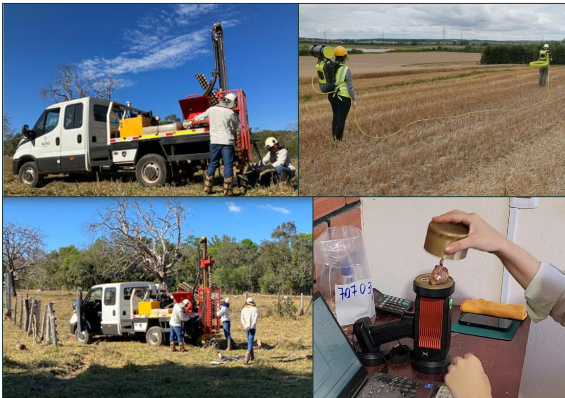
Figure 5: Alvo's auger rig drilling at Bluebush REE Project (Boa Vista Prospect Top left and bottom). Loupe Electromagnetic equipment in action (not from Alvo's areas- see Loupe Geophysics – New Technology in Portable TEM for Near Surface Measurements. ) SciApps X-555 portable XRF analyzer in action at Alvo's core shed.
