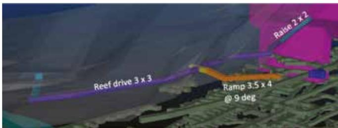
**Figure 6: Access ramp, reef drives/first cut at the +105 trial mining project**
