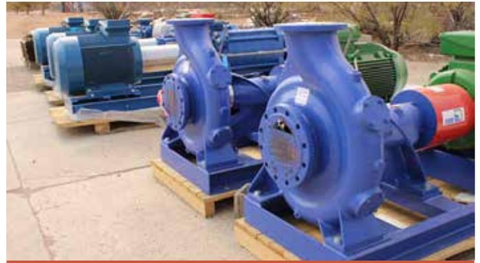
Figure 3: Multi-stage dewatering pumps
