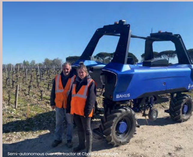
Semi-autonomous over-row tractor at Chateau Tanessan
