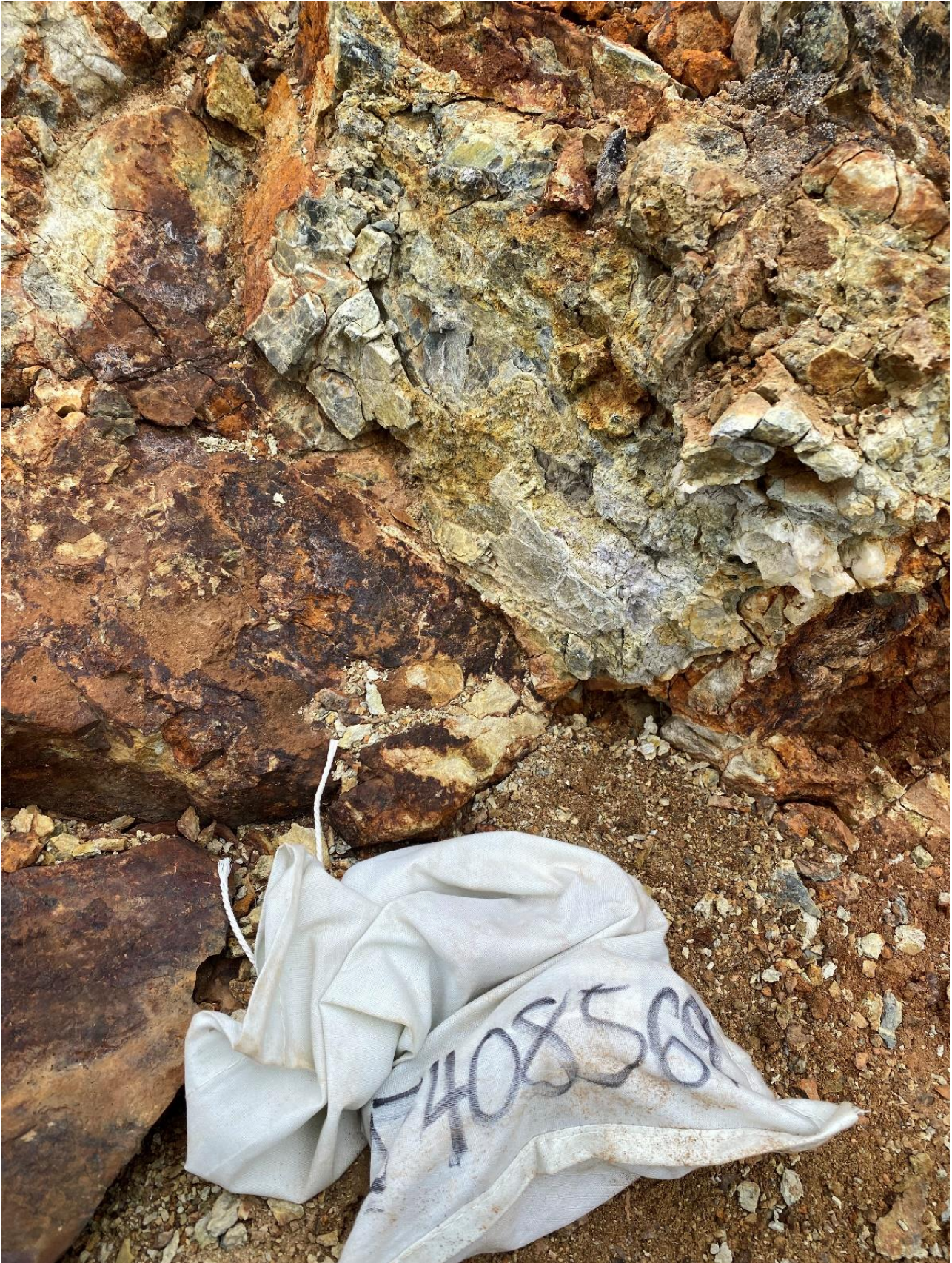
Figure 3. Mineralized quartz vein ~2m wide and exposed on surface with over 30m strike containing abundant sulfides including Arsenopyrite and Stibnite, found on the new claim area
