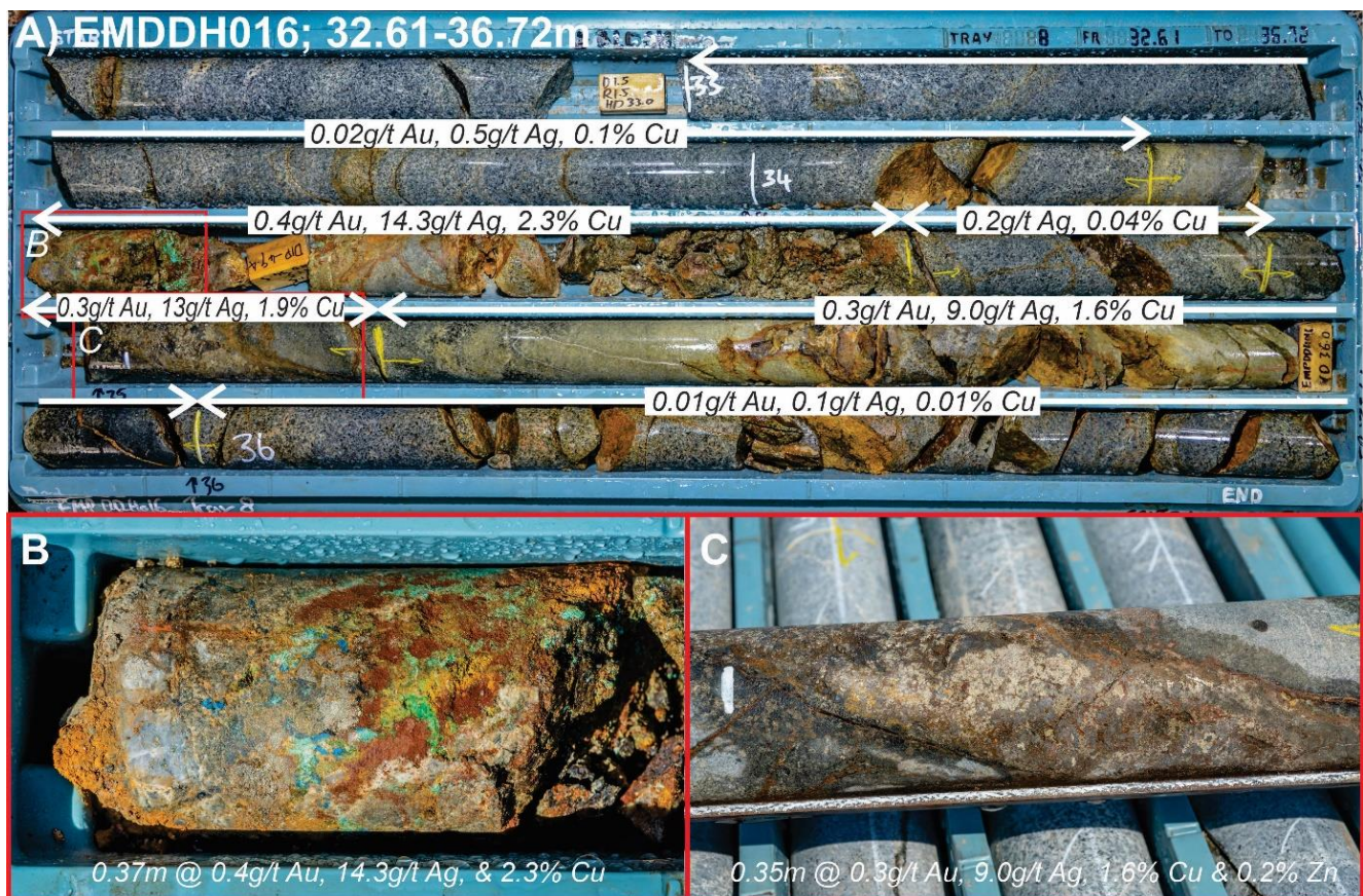
Figure 6 – Core tray from EMDDH016 from 32.61-36.72m showing Ag-Cu mineralised interval with trace Au. A) Core tray image showing assay results for Au, Ag, and Cu. B) Zone of oxidised sulphides with abundant iron and copper oxides, including malachite (green) and azurite (blue). C) Sulphide vein comprised of pyrite, chalcopyrite, and sphalerite.
