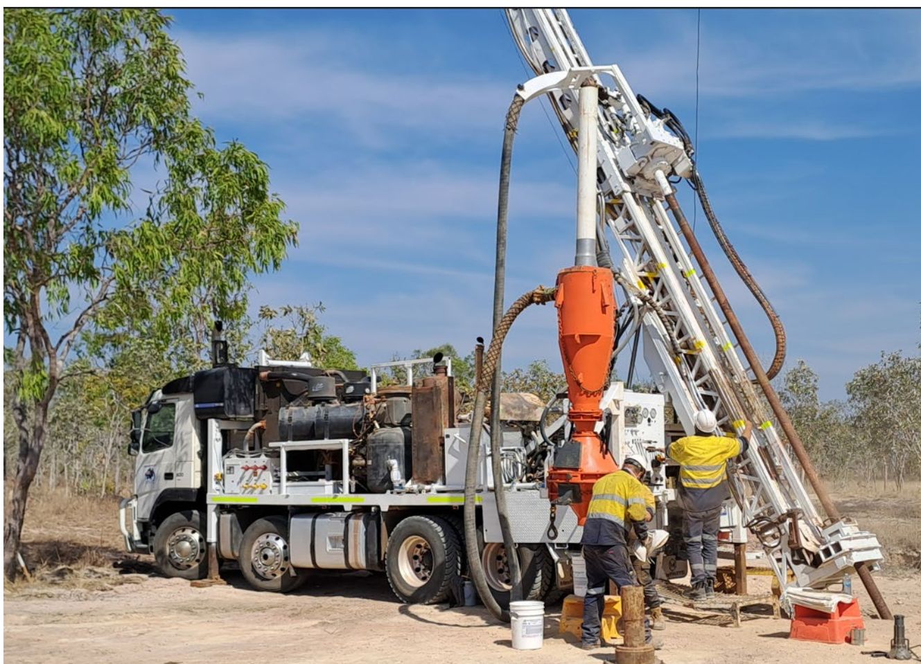
Figure 2: RC drill rig (UDR650) at Posie prospect which is the first drilling to be undertaken at Posie for 30 years.
