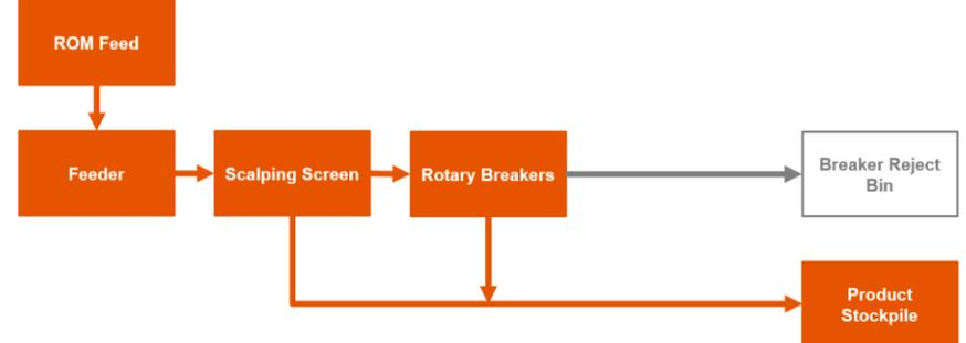
**Figure 9: General flow of the ROM circuit at Blackwater TCP**
