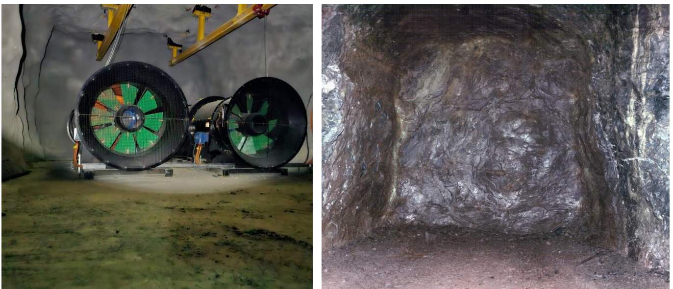
Figure 2: Xantho Extended booster fans (left). Development face in the high-grade zinc Xantho Extended orebody (right).
