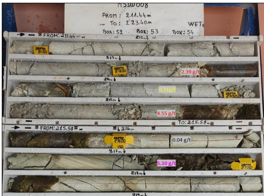
Figure 6: MSDD008 Showing intersection of 5m @ 2.5 g/t gold from 213m, with distinct hematite + chlorite selvage around massive and brecciated qtz+py veins.
