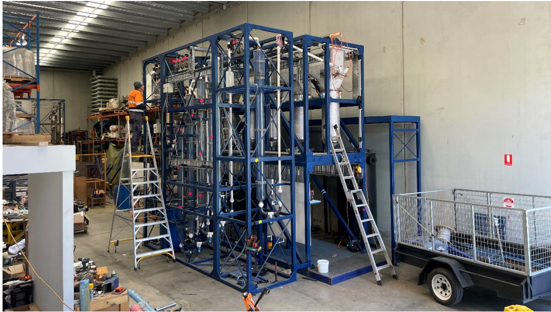
Clean TeQ's cDLE ® demonstration plant being prepared for shipment to Lithium Bank
