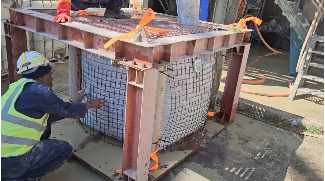
ATA ® solids in geotextile bag being dewatered in South Africa
