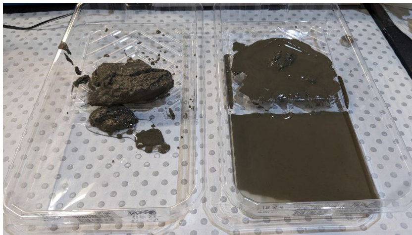
Testwork for an Australian mine showing ATA ® solids (left) vs their current flocculant (right)
