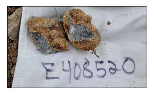
**Figure 2.** Sample E40820 - **1,290** g/t Au, 0.9% Sb, 591 g/t Ag, 1.0% Cu, 1,300.1 g/t AuEq talus sample collected in chute
