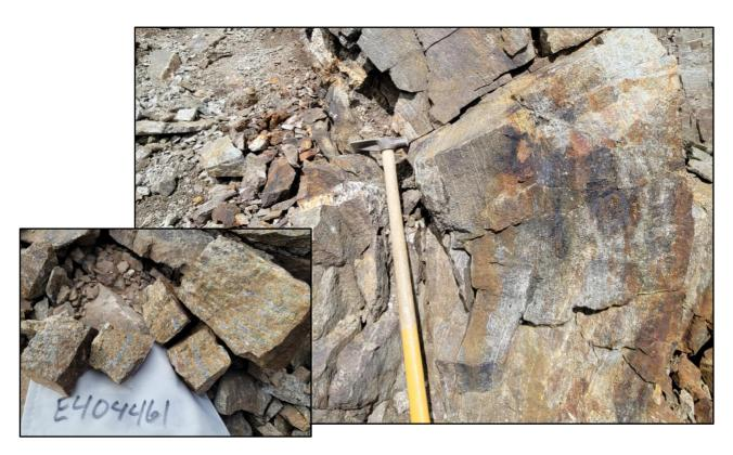
Figure 3. Outcrop sample E404461 – 35.6 g/t Au, 1.0% Cu
