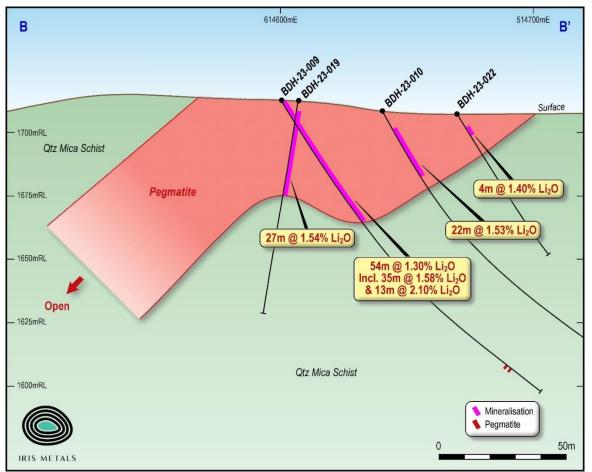
Figure 3: Cross section showing reported lithium intersections.
