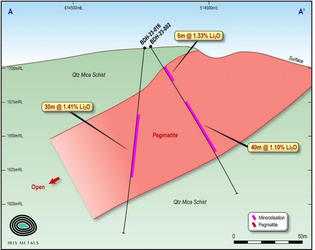
Figure 2: Cross section showing reported lithium intersections.
