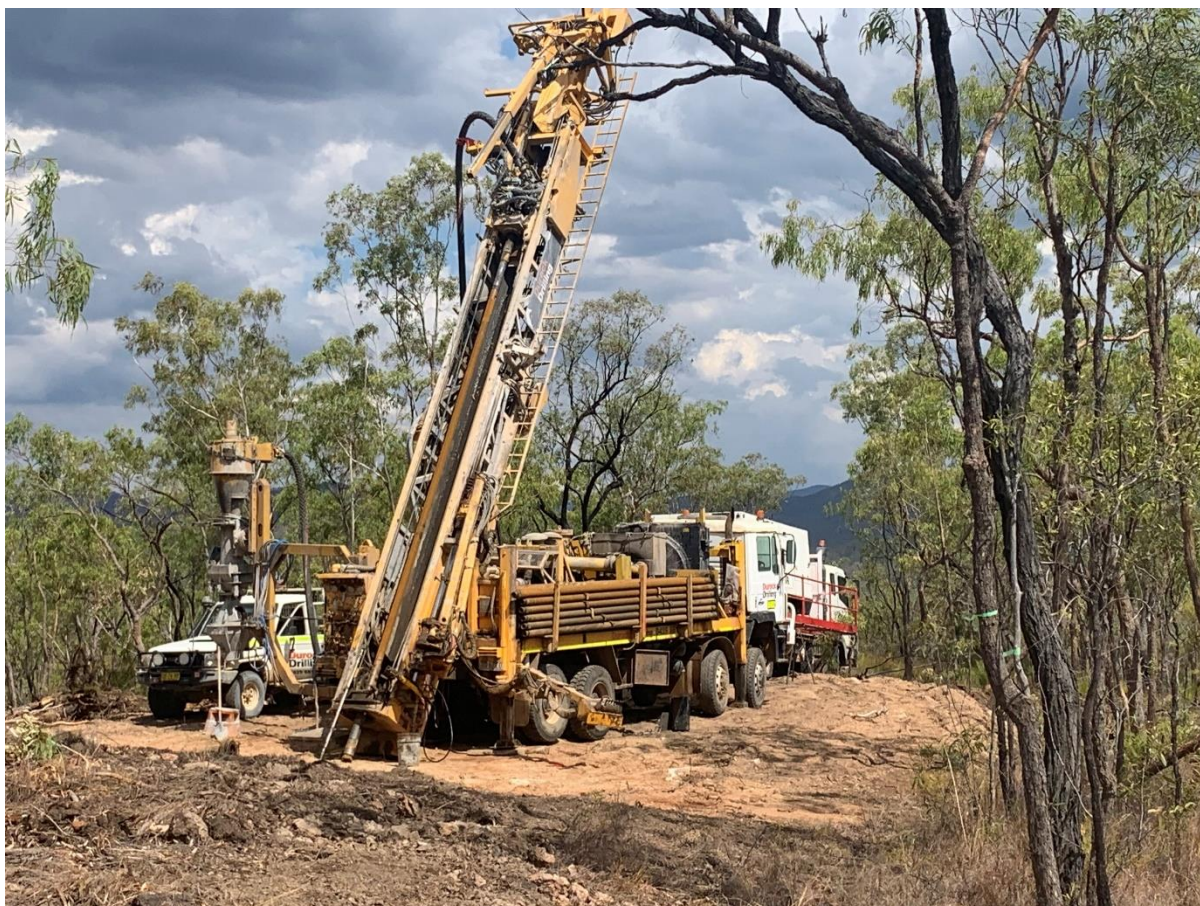
Figure 1 RC Drill Rig at Orient East
