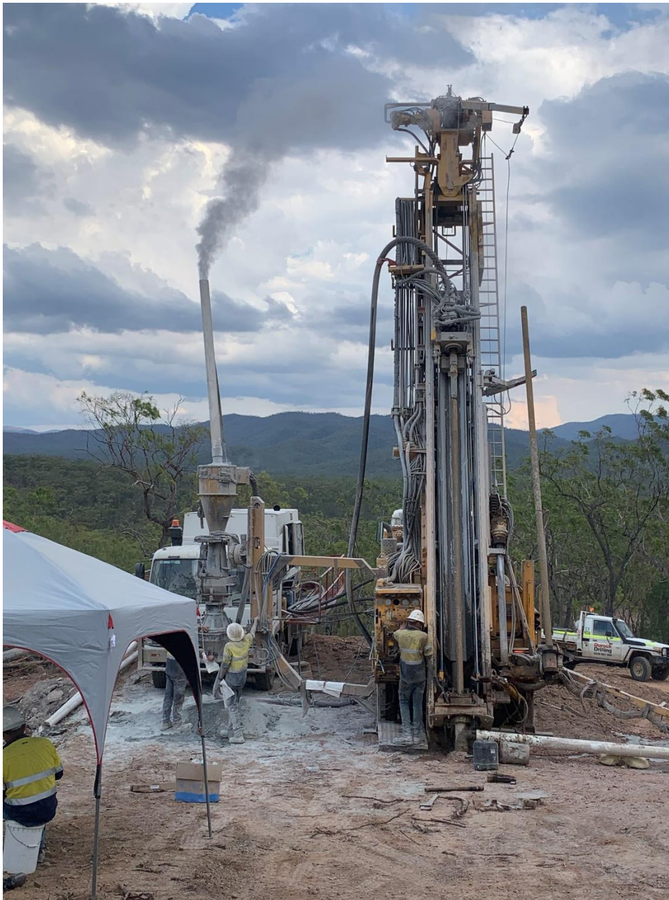
Figure 2 Stage 2 RC drilling at Orient Project
