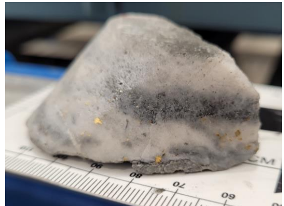
Photos 3 a & b: SDDSC082 from 418.6 m (within assayed interval 0.2 m @ 4,190 g/t AuEq (4,190 g/t Au, 0.1% Sb) from 418.4 m to 418.6 m) showing visible gold within and quartz-carbonate and stibnite vein. Millimetre scale.
