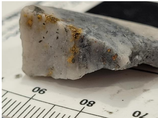
Photos 3 a & b: SDDSC082 from 418.6 m (within assayed interval 0.2 m @ 4,190 g/t AuEq (4,190 g/t Au, 0.1% Sb) from 418.4 m to 418.6 m) showing visible gold within and quartz-carbonate and stibnite vein. Millimetre scale.
