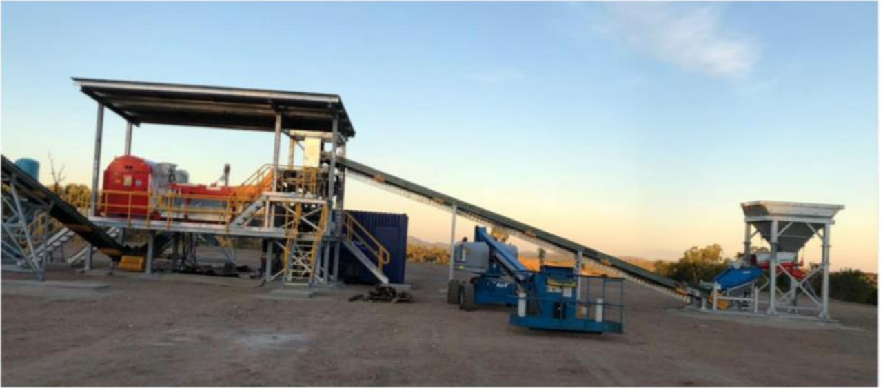
Figure 6. Bulk test pit conceptual ore sorter image
