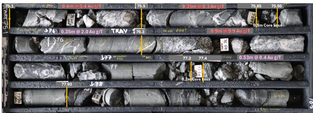
Figure 4 – Photographed core from DNDD001 showing high grade gold intervals in lode style quartz veins from mineralised zone 7.2m @ 2.5g/t Au from 68.9m.
