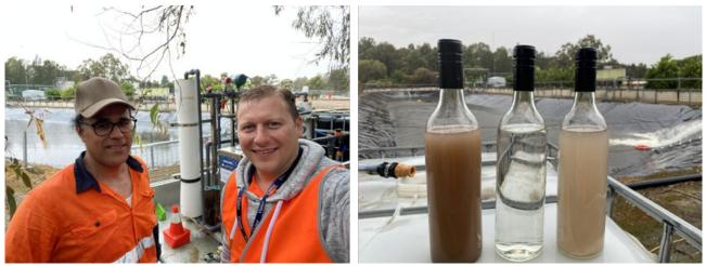
Left Image: Dr Abozar Akbari and Dr David Menzies onsite running the beverage wastewater pilot Right Image: Water produced during the pilot – Retentate (left), Permeate (center) and feed (right)
