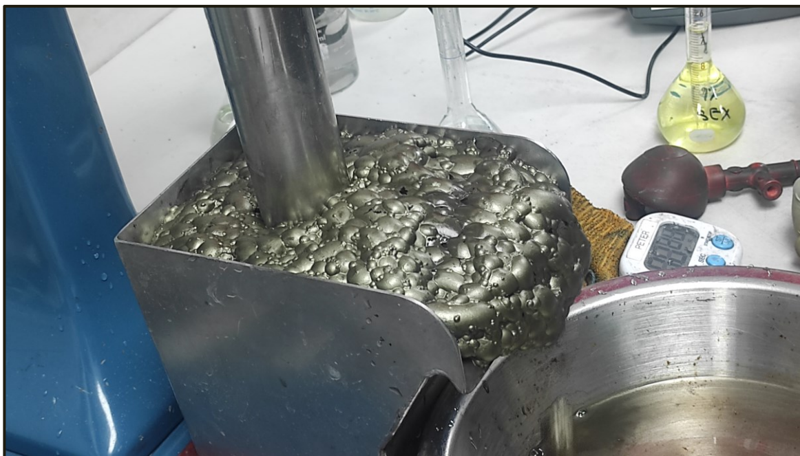
Photo 6: Photograph showing a batch flotation test of the PCZM supergene ore at Maelgwyn.
