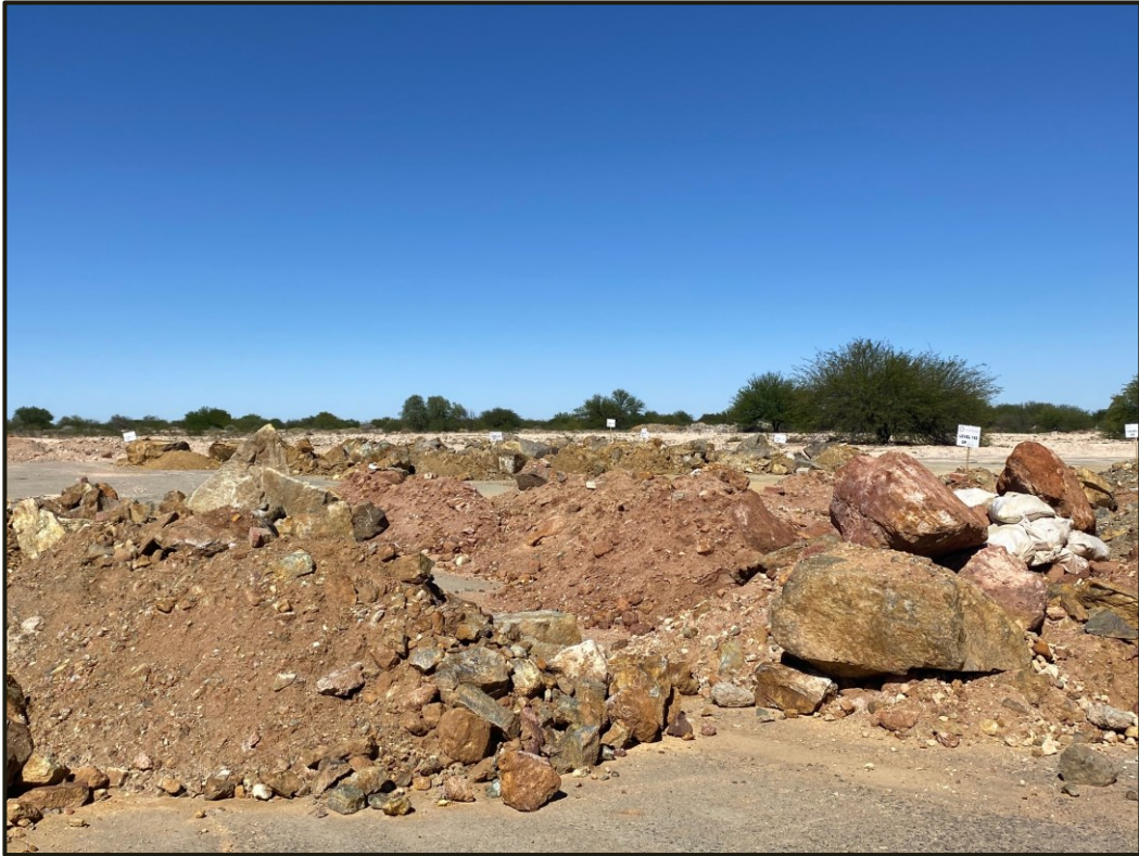
Photo 2: 143 Level drawpoint material stockpiled on surface.
